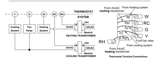
Figure 8. Typical Wiring Diagram for Heat/Cool, 5-Wire, Two-Transformer System
